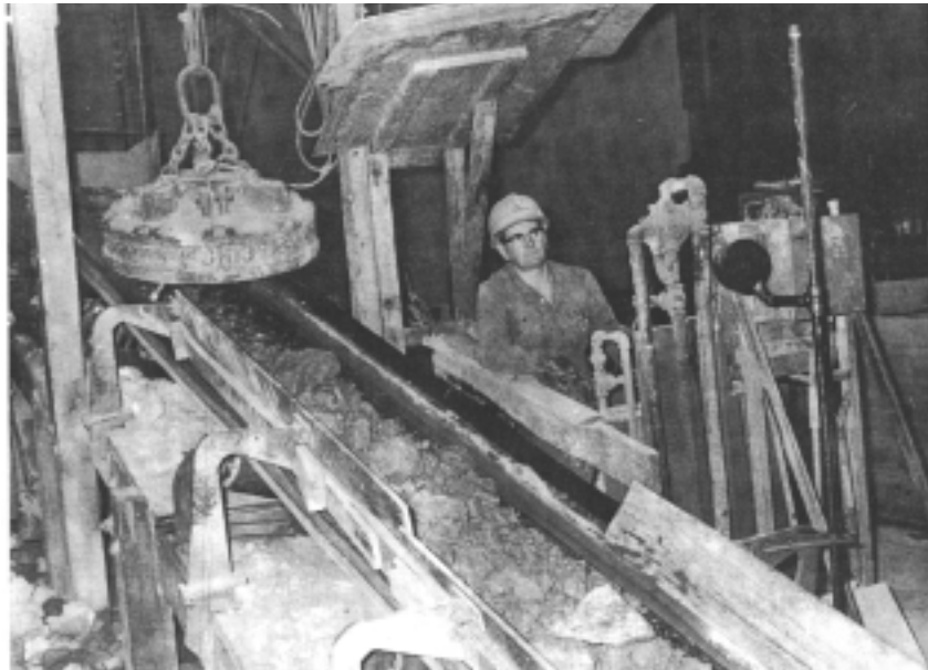
Bob Burley operates jaw crusher that removes metal objects from chunks of ore
